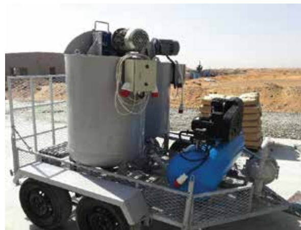
Pos. 3 ECOCON 2X9 bags mixer (450 kg mixing batch)
