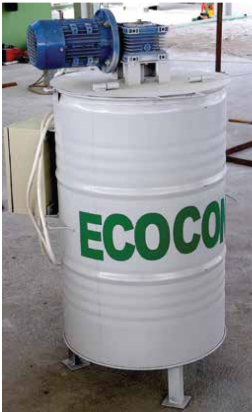
Pos. 2 ECOCON 3 bags mixer (150 kg mixing batch)
